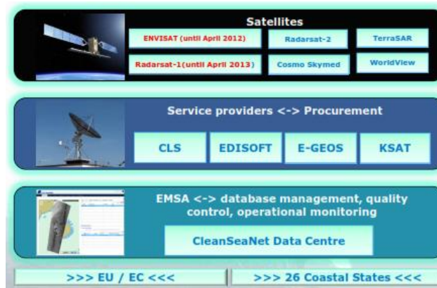
Figure 4. EMSA CleanSeaNet system - Architecture
